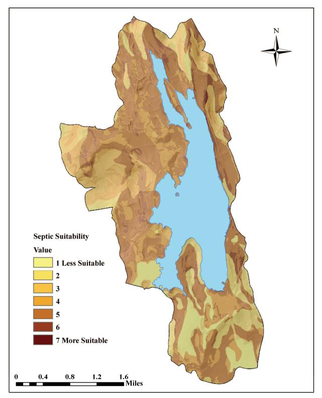
Figure 22. A model showing septic suitability of the Long Pond North watershed which combines soil suitability and slope into an index of 1 (low suitability) through 7 (highly suitable). The index is based on soil type and degree of slope.
