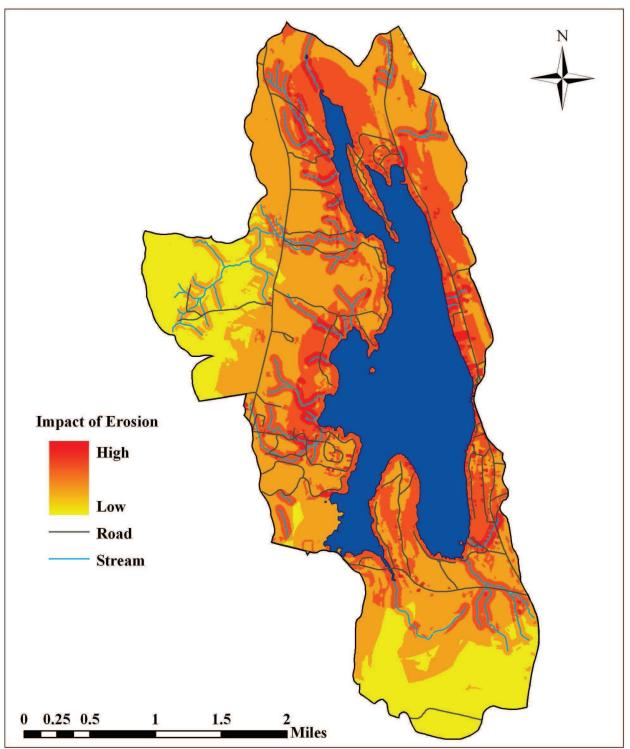
Figure 26. Impact of erosion map for the Long Pond North watershed. The impact of erosion was determined by combining erosion potential ratings with proximity to Long Pond North or one of its tributaries. Areas where erosion is likely to have a high impact on Long Pond North water quality are shown in red, and areas with a low potential impact of erosion are yellow. The streams and roads layerswere obtained from the Maine Office of GIS (MEGIS 2006).
