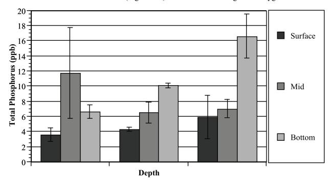
Figure 42. Mean (± SE) surface, mid, and bottom phosphorus concentrations (ppb) in 2006 for Long Pond North site 1 (see Figure 28 for site locations). Italicized values in Appendix C were omitted.
