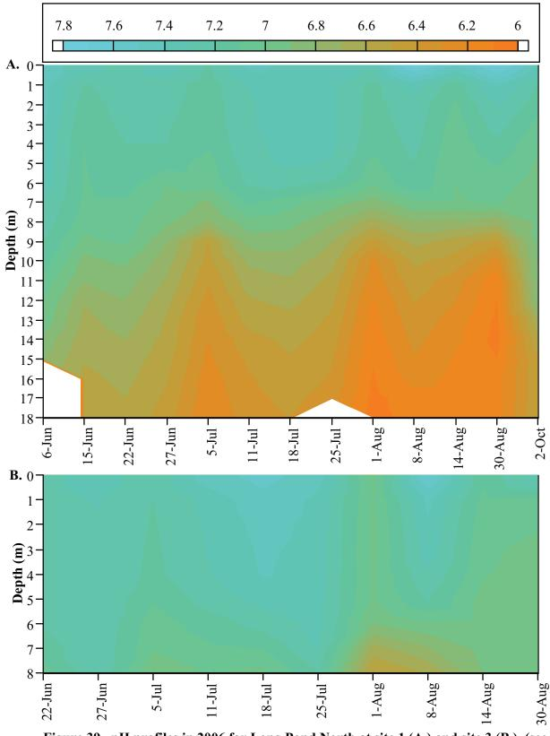
Figure 39. pH profiles in 2006 for Long Pond North at site 1 (A.) and site 3 (B.) (see Figure 28 for site locations).
