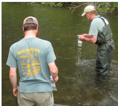
CASWCD and Maine DEP staff collect water samples to determine turbidity
