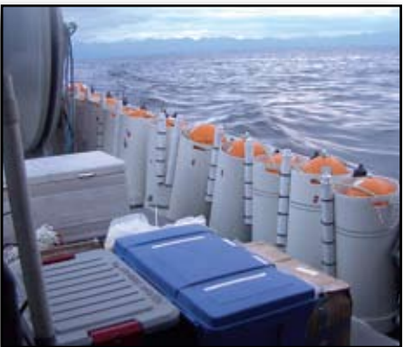
An acoustic unit being deployed in a test. Each unit has a yellow flotation device, white acoustic modem and black acoustic receiver.
