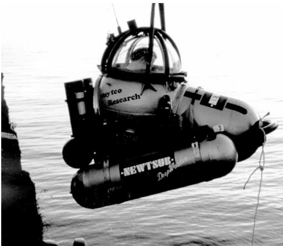
Newtsub DeepWorker 2000, a submersible developed by Nuytco Research Ltd. in Canada, will be used during the Sustainable Seas Expeditions, allowing exploration of the ocean down to 2,000 feet/610 meters.
