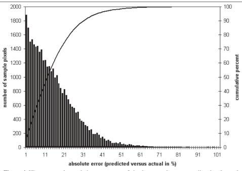
**Figure 4.** Histogram and cumulative percentage of absolute error between predicted and actual percent imperviousness using sampled pixels from the Chesapeake Bay study area.
