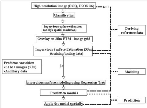
**Figure 1.** The proposed procedure for impervious surface mapping using Landsat-7 and high spatial resolution imagery and a regression tree model.
